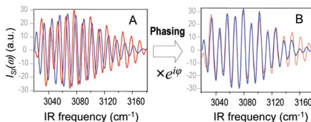
**Figure 3.** Phasing procedure allowing us to lock the phase of the SI to that of the background signal of the neat (fully deuterated) interface. (A) Real parts of the SI from 10% octanol monolayer sample (red line) and neat interface (blue line) before phasing in the spectral region around  $3100 \text{ cm}^{-1}$ . (B) Same two SI after phasing (red interferogram multiplied by  $e^{i\phi_{\text{adj}}}$ ).
