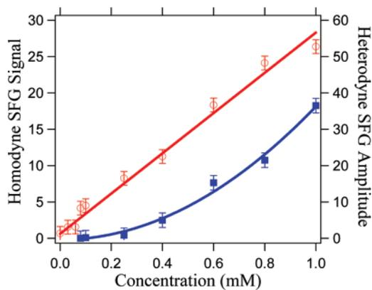
**Figure 6.** Scaling of the homodyne-detected SFG intensity (blue squares) and HD-SFG signal amplitude (red circles) with the surface coverage (1-octanol mol fraction in the monolayer) for the CH<sub>3</sub> symmetric stretch mode.
