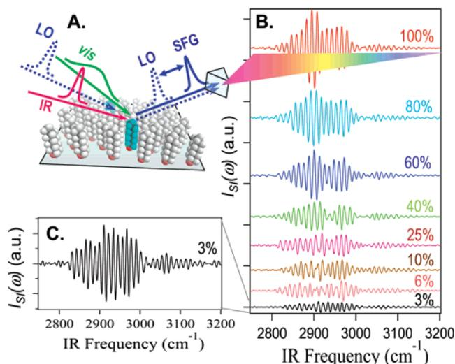
**Figure 1.** (A) Schematic representation of the broad-band heterodyne-detected HD-SFG experiment. (B) SI (real part shown) for samples of varying surface coverage of 1-octanol, from 100 to 3% monolayer. (C) Enlargement of the signal from the 3% monolayer sample.
