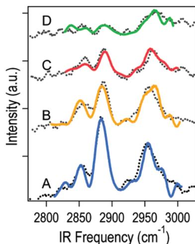
**Figure 2.** Comparison of the power spectra of 1-octanol CH-stretch vibrations obtained from the heterodyne-detected spectral interferograms (thick colored lines) with the conventional (homodyne-detected) SFG spectra (black dashed lines) for surface coverages of (A) 100%, (B) 80%, (C) 60%, and (D) 40% monolayer.
