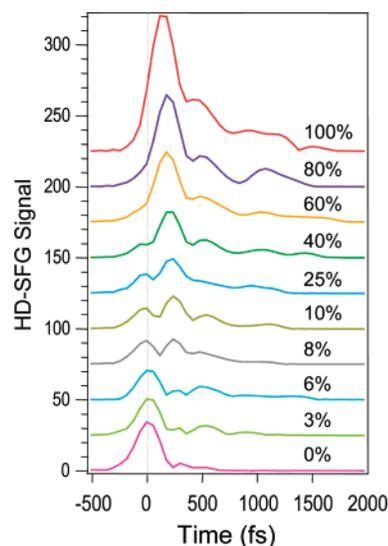
**Figure 5.** Time-domain vibrational free induction decays at various 1-octanol mol fractions in the monolayer, showing vibrational quantum beats of the CH-stretch modes of 1-octanol and the background response of the neat (0%, fully deuterated) interface consisting of both non-resonant components peaking at  $t = 0$  and resonant vibrations of impurities ( $\leq 2\%$  level).
